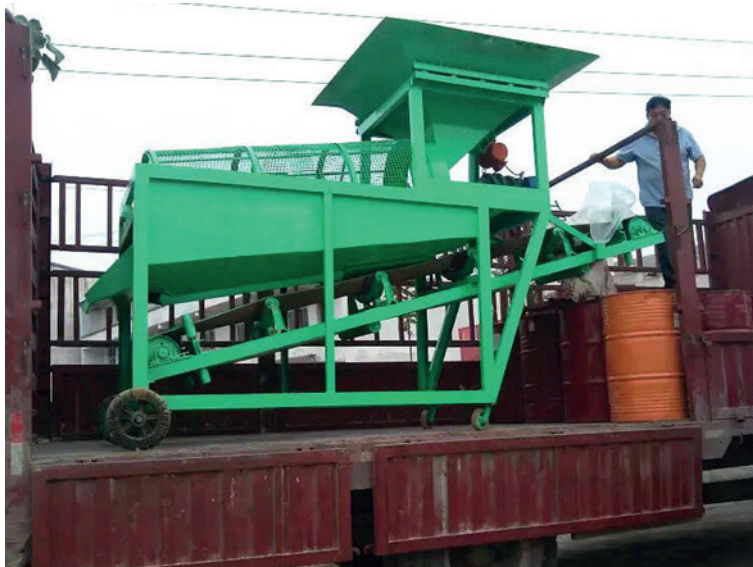
Figure 8: Example of a sand sieve machine for cleaning 'dirty' sand sources.
